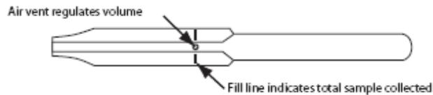
**NOTE:** Once the specimen is drawn into the sample transfer pipette, the pipette will not leak; the pipette will hold the specimen until the bulb of the pipette is squeezed.
