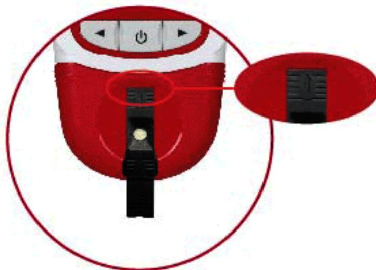
Ensure that the test cartridge is inserted all the way to the end of the cartridge channel.
