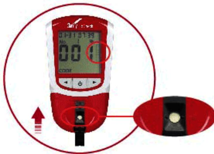
**Note: Insert the cartridge without bending it.**
