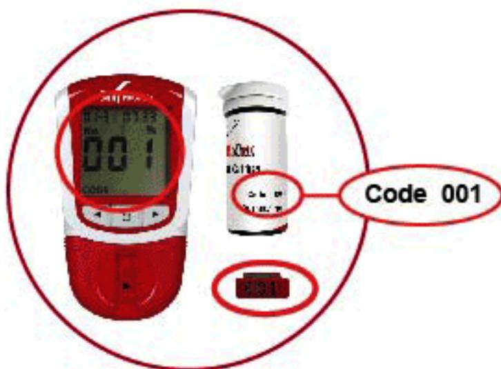
Make sure the code on the display matches the code number on the test cartridge canister label and on the code chip.
