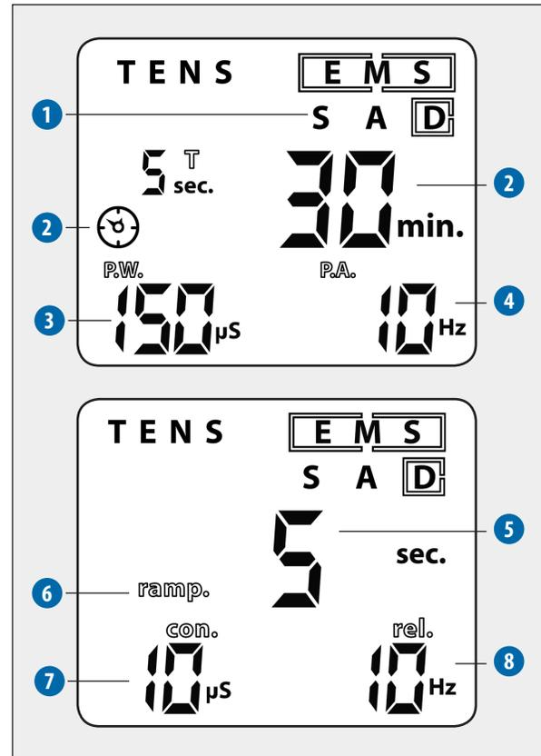
**Caution: Contract time does not include the ramp up and ramp down time, ON time = Ramp up + Contract time + Ramp down.**
