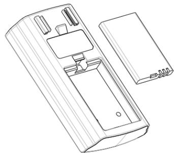
Press down on the belt clip to release it. Remove the battery cover and insert the battery as shown in the diagram. Replace the battery cover and belt clip.
