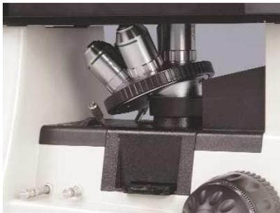
*Close-up of the inverted nosepiece and objectives.*
