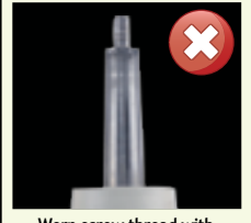
Worn screw thread with non genuine ACTEON® EQUIPMENT tips
