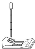
5. Dispense all of the solution in the transfer pipette into the Extraction Well of the test device.
