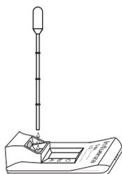
2. Dispense the entire sample in the transfer pipette into the Extraction Well of the test device.
