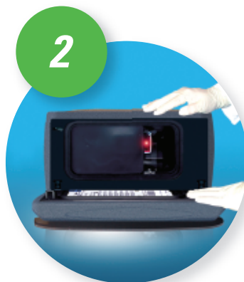
2 Place FastPack® into the FastPack® IP Instrument
