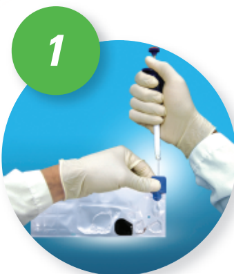
1 Dispense sample into the FastPack® Injection Port
