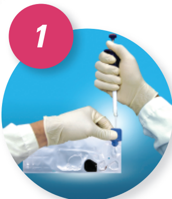
1 Dispense sample into the FastPack® Injection Port
