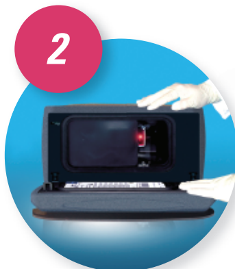
2 Place FastPack® into the FastPack® IP Instrument
