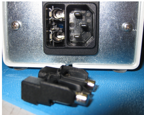
Figure CM-01, Fuse Holder
