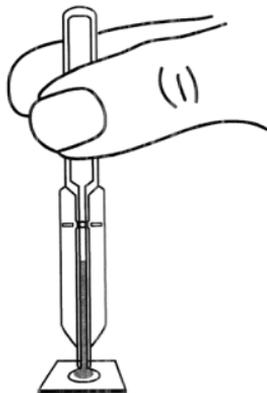
**Step 2:** To expel the sample, align the tip of the tube with the sample target and squeeze the bulb.
