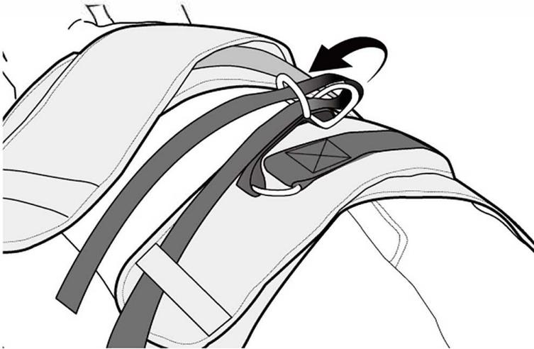
*BRING* the open end over the second ring then *INSERT* through the first ring. *PULL* the open end to increase tension.
