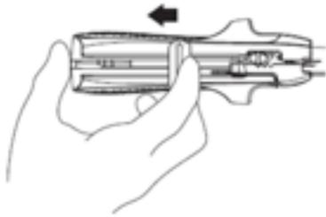
If Firing Knob is not in "RETURN KNOB HERE" position, return the Firing Knob to the original prefiring, "RETURN KNOB HERE" position.
