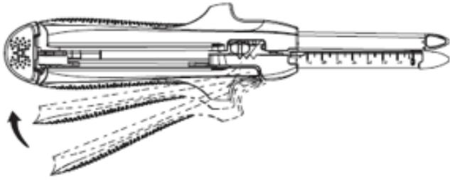
Ensure that the Cartridge/Reload Fork and the Anvil Fork are aligned. Close the Alignment/Locking Lever completely when the tissue is properly in place.
