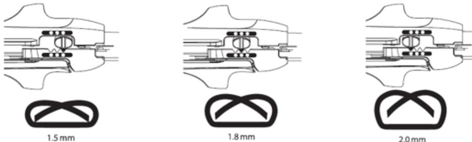
Prior to placing instrument across the tissue, select the desired closed staple height. In order to select the desired staple height, push the Staple Height Selector so that it is aligned with desired color indicator, Blue 1.5 mm, Gold 1.8 mm or Green 2.0 mm. If tissue cannot be comfortably compressed to the closed staple height, or easily compresses to less than the closed staple height, either the setting or the tissue is contraindicated for the selected staple size or setting.
