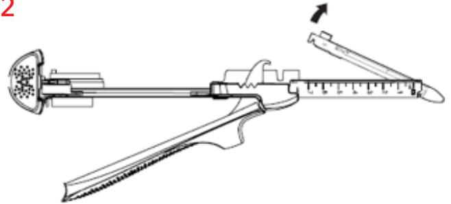
Separate the instrument halves by pulling open the Alignment/Locking Lever. Pull upward on the Gripping Surface and unsnap the used Cartridge from the Cartridge Fork. Discard the used Cartridge.
