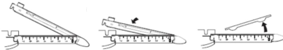
Examine the new Cartridge for the presence of a Staple Retaining Cap. If the Retaining Cap is not in place, discard the Cartridge. Insert the new Cartridge by placing the Alignment Tabs into the Alignment Slots and pivoting the Cartridge into the Cartridge Fork. Snap the Cartridge into position. Remove the Staple Retaining Cap and discard.
