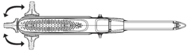
With the instrument closed, the Firing Knob is rotated to either side of instrument.
