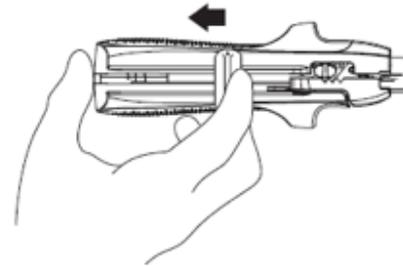
Completely return the Firing Knob to the original pre-firing, "RETURN KNOB HERE" position.
