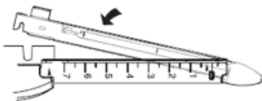
Load the instrument by inserting the selectable Cartridge/Reload by placing the alignment tabs into the alignment slots and pivoting the selectable Cartridge/Reload onto the Cartridge/Reload Fork. Snap the Cartridge/Reload into position.
