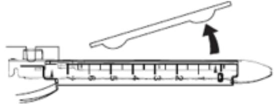
Remove Staple Retaining Cap by grasping the edge of the Staple Retaining Cap and lift straight up from the Cartridge/Reload. Discard the Staple Retaining Cap.
