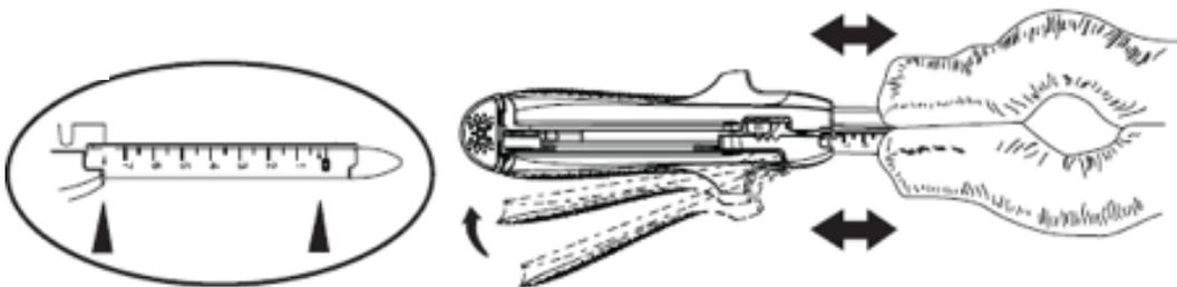
**CAUTION:** When positioning the device on the application site, ensure that no obstructions such as clips, stents, guide wires, and etc., are within the instrument anvils. Firing over an obstruction may result in incomplete cutting action and/or improperly formed staples.
