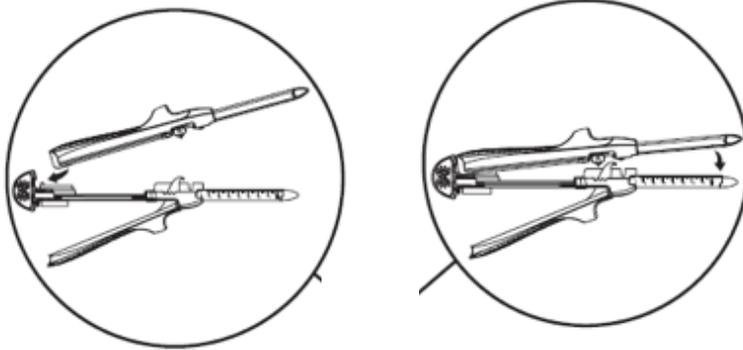
With the Alignment/Locking Lever in the completely opened position, join the instrument halves together by aligning from either the front, center, or back of the instrument. To adjust tissue on the forks before firing, move the Alignment/Locking Lever to the intermediate position. This allows maneuvering of the tissue while the instrument halves are joined.
