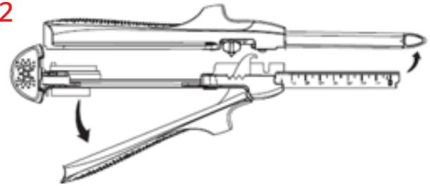
If instrument is not separated into halves, separate instrument by completely disengaging the Alignment/Locking Lever.
