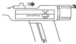
Open the instrument by rotating the Adjusting Knob counterclockwise. (The Retaining Pin may be pulled back to its original position to facilitate instrument removal.)
