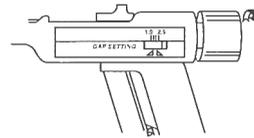
Open the Jaws completely by rotating the Adjusting Knob counterclockwise, until it stops.
