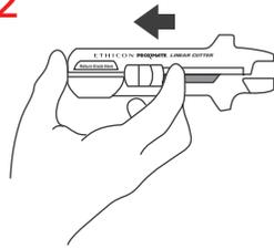
Completely return the Firing Knob to the original "Return Knob Here" position.
