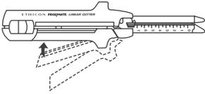
Close the Alignment/Locking Lever completely when the tissue is properly in place.
