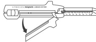
Separate the instrument halves by opening the Alignment/Locking Lever and remove the instrument.
