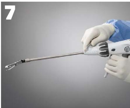
To articulate the jaws inside the body cavity, turn the articulation lever in either direction until one of the three pre-determined angles is reached. **Articulating while closed does not provide optimal feedback and control**, and may result in instrument damage.
