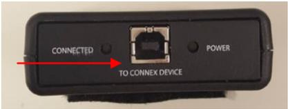
2. Connect the other end of the 6.6ft USB cable to any available USB port on the Welch Allyn Connex monitor.
