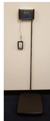
2. Connect the other end of the 1ft. USB cable to the USB port on the display head.
