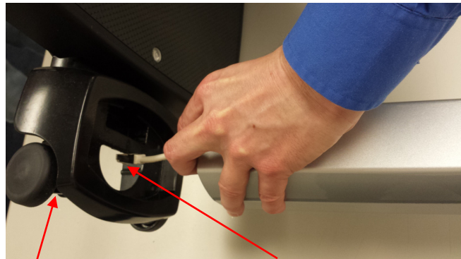
Load Cell Cable Connector
