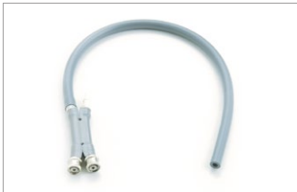
Wall Manometer Adapter only Includes adapter with female screw connector and 13" tubing (no coiled tubing, no bulb and valve) Part # 330076 (10/Pk)
