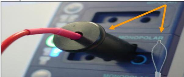
6. Plug the Grounding Pad into the NEUTRAL receptacle and place the Pad on the patient.
