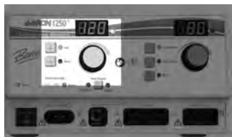
Figure 2 – 2 Controls for the Cut and Blend Modes
