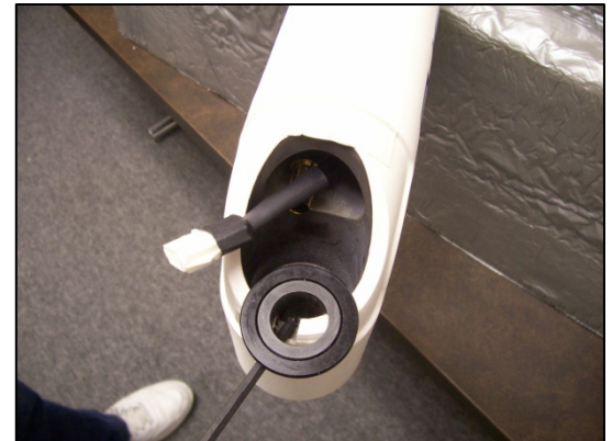
24. Install plastic bearing first.
