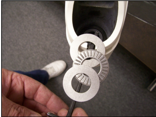
25. Install Thrust bearing components by passing the cables one at a time through each component.
