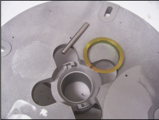
13 a. Ceiling Casting b. Tapered Collet c. 3.5" long Dowel Pin.
