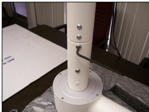
5. Use four 5/16 screws to mount Extension Arm Assembly to Ceiling Extension Rod.
