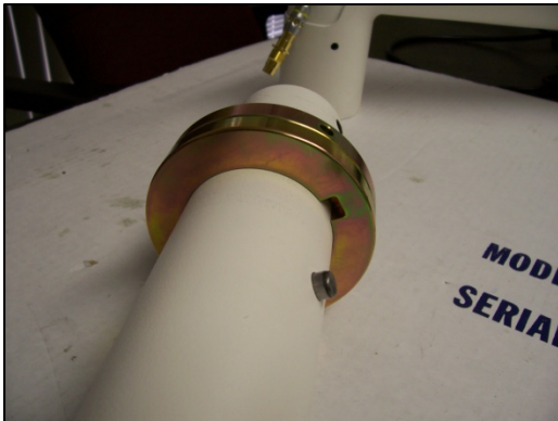
10. Jack Screw rings on Extension Rod. Mate notch on lower Jack Screw ring with Dowel Pin.
