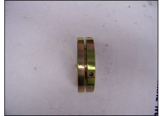
9. Jack Screw rings assembled.
