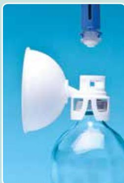
The Protector is a pressure equalization device, permanently attached to the vial used in the preparation of drugs from either powder or liquid form. When attached to a vial, the Protector provides closed pressure equalization through the sealed expansion chamber and dry connections via the double membrane design. This ensures that there is neither overpressure nor vacuum when air or fluid is injected into or aspirated from the vial.
